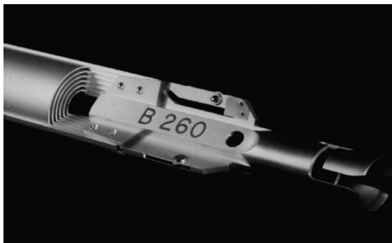
Fig. 1. Standard BR2 element consisting of six concentric tubes, each tube being an assembly of three equal curved segments (plates). In the described irradiation program six \text{U}_3\text{Si}_2 fuel plates constitute the outer cylinder of two standard BR2 elements.
